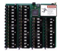
On the inside of the TRACKER unit, you will find a single printed circuit board with one (1) 3-pin connector on the top center just above the microprocessor, one (1) 2-pin connector by the power supply, and forty-eight (48) 2-pin connectors in four columns.
